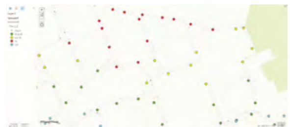
Figure 4: Fire hydrant performance mapping.
