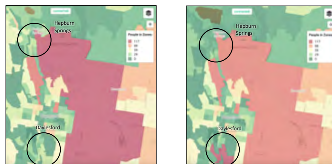
Figure 3: SEEKER output showing change in number of people in Hepburn Springs and Daylesford (black circles) between 6pm Feb 2 (left) and post-evacuation at 10am Feb 3 (right).
