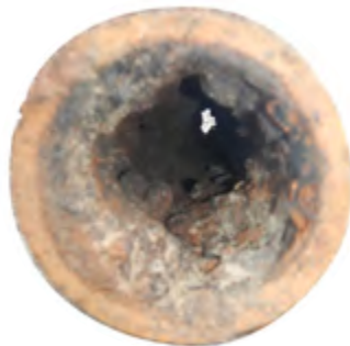
Figure 1: photograph of a cement lined in-situ pipe
