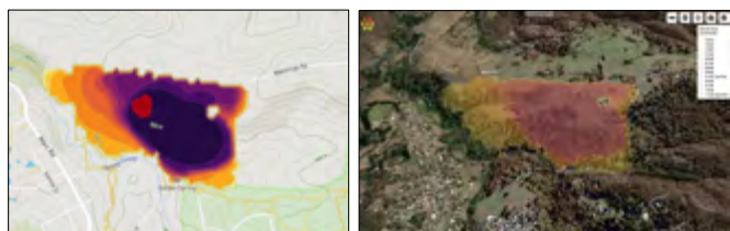
Figure 2: The final SPARK arrival time isochrones for the predicted fire run. Left: Illustration of the isochrones on a 2D topographic map. Right: Isochrones overlaid on 3D satellite imagery.
